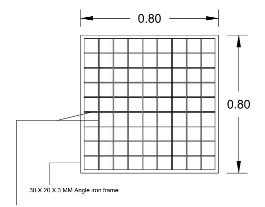
5 MM Dia M.S. rods for net @ .085 M c/c
